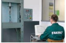
Testing resistance to tearing
