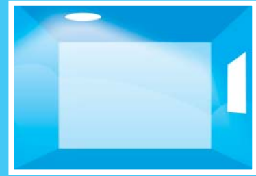
light tunnel placement in a room with a window. The placement of a light tunnel too close to a wall opposite to a window may diminish the overall light in the middle zone.
