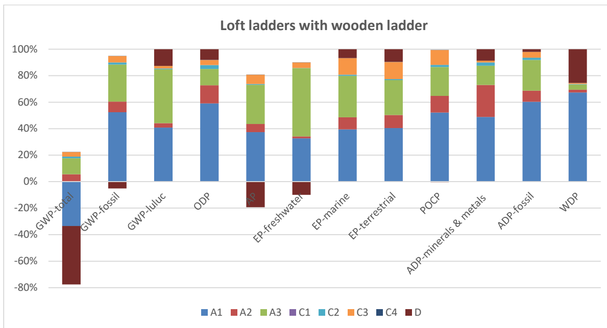
Figure 3 Shares of life cycle modules on the main categories of influence – loft ladders with wooden ladder.
