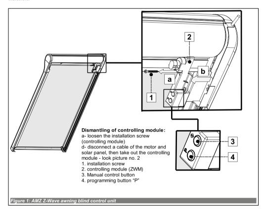
In the AMZ Z-Wave awning blind the ZWM controller is located under the right-side body cover - see *Figure 2*.
