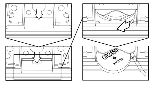
3. Put the battery into position paying attention to the correct polarisation. Position the tape for removing the battery in a way enabling sliding the battery out again with the use of this tape.
