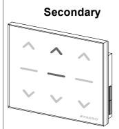
4. After few seconds, the controller is signalizing that associating with the network has been successfully completed (buttons light up for 2-3 sec. as presented in the drawing).
