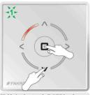
Hold simultaneously DOWN and STOP buttons until one of LEDs starts blinking.
