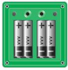
Place the batteries as shown in the picture before you start using the ZRW7 control keypad.
