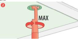
Place the tip of the rod in the catch recess on the hatch.
