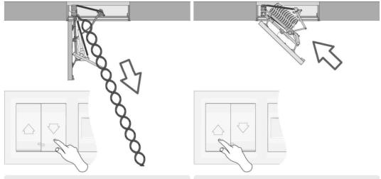
Hold the "DOWN" button to open the LET type loft ladder.
